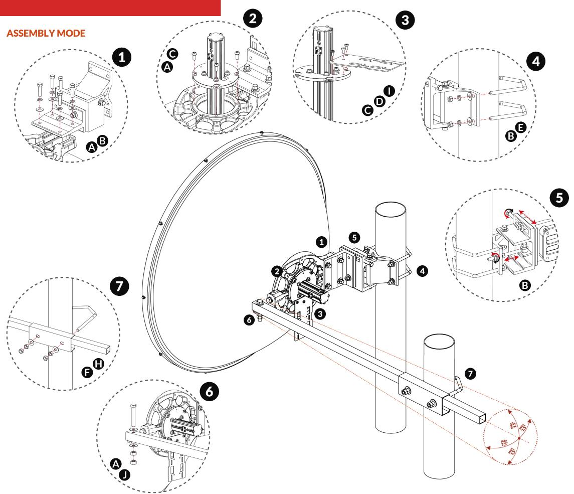
Assembly of the model UHP-5800-32-09-DP. Image dimensions may be different in size.
